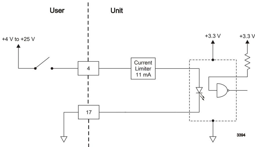
Figure 4-4. RF PWR ON (pins 4 and 17)
