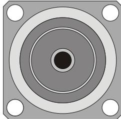
*Figure 5-9. RF output connector, HN coaxial, female (TRU-8371-SNT)*
