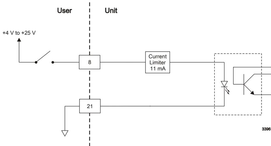
Figure 4-7. FWD/LOAD PWR REGULATION (pins 8 and 21)
