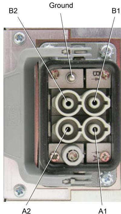
**Figure 5-10.** HARTING AC 70 A power input connector on back of unit
