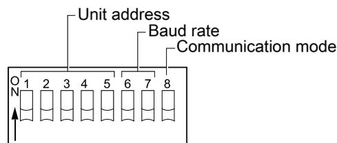
**Figure 4-14.** Slide DIP switch
