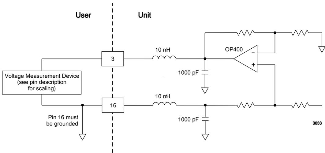
Figure 4-3. FWD/LOAD PWR MONITOR (pins 3 and 16)
