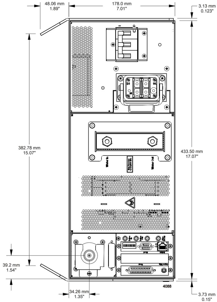
Figure 5-3. Rear panel with dimensions
