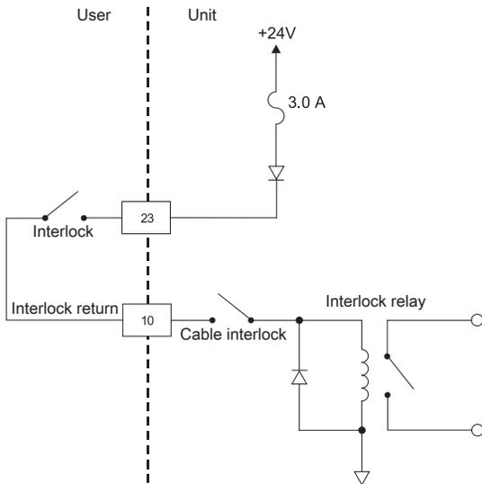
Figure 4-8. INTERLOCK LOOP (pins 23 and 10)
