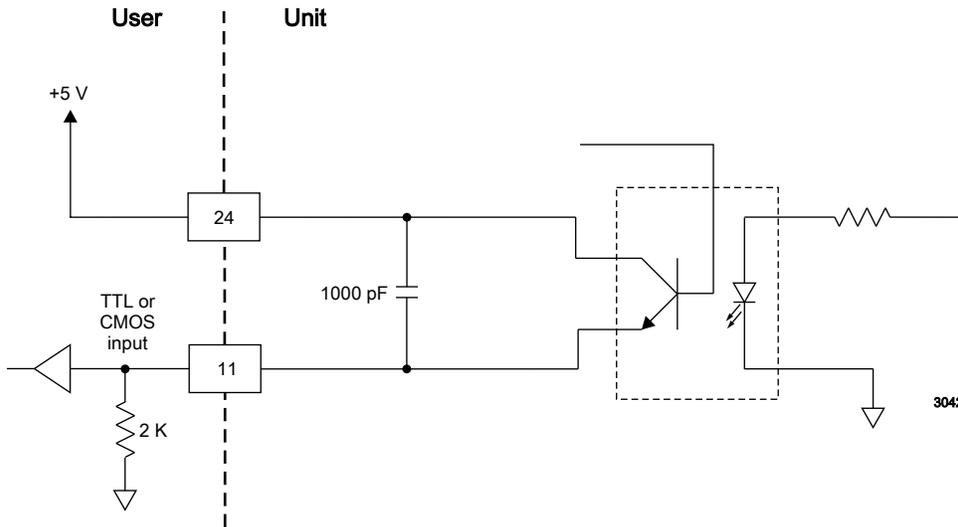
Figure 4-12. DC BUS OK (pins 24 and 11)
