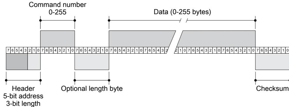
Figure 4-15. Graphic representation of a message packet
