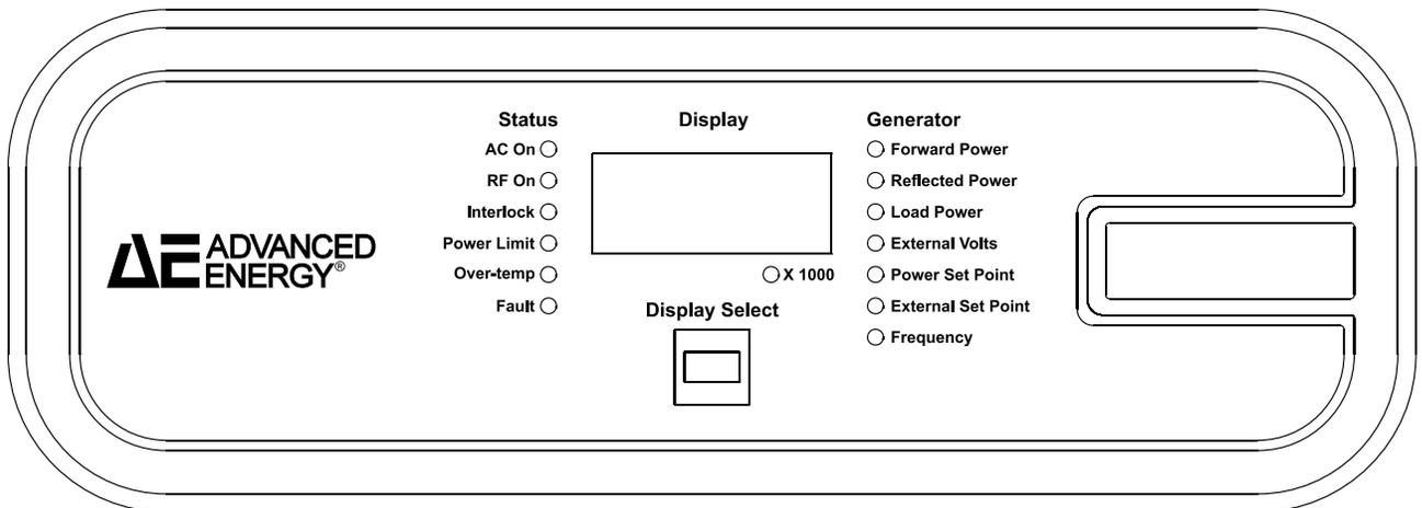
**Figure 5-11.** Front panel display with Status and Generator LEDs
