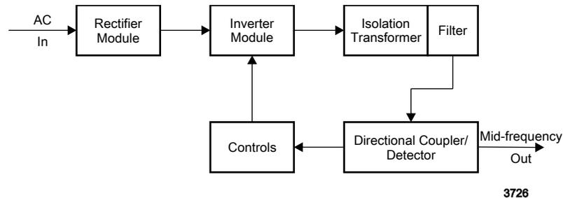
*Figure 2-1. Paramount MF 2 kW generator block diagram*
